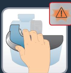
**EN** Remove the dust container by lifting it upwards. The
