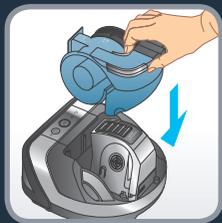
**EN** Put the dust container back into the robot. The
