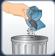
**EN** Press the button « PUSH » to open the container and empty it.
