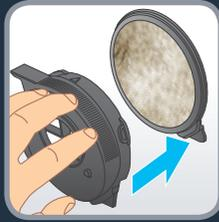
**EN** Once a week, wash the filter with clear water and clean the dust container and the cyclone manually.
