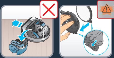
**EN** The robot will not start if the dust container or the filter is missing. In that case, the error light will be lighted fixed and the dedicated message will be displayed on the app.
